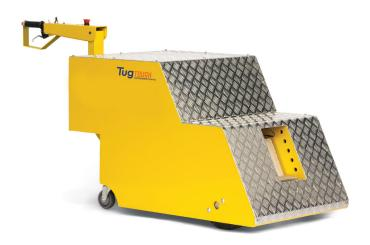
The perfect heavy duty workhorse for loads up to 10 tonnes, the Tug Tough utilises a powerful 48 V drive system to allow a single operator to hitch to and move big loads.
