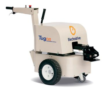
A powerful machine, the Tug Evo is available in one or two tonne towing capacities.
