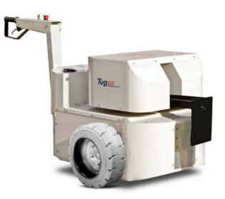
The Tug Rise pedestrian operated electric tug has been designed to tow on slopes or ramps, and is capable of towing up to 1 tonne on a 15 degree ramp with ease, or up to 5 tonne on a flat surface.
