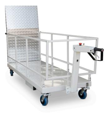
The Powered Bin Trolley can move up to three 240 litre wheelie bins—weighing up to 400 kg over a flat surface. Its powered drive-wheel can also handle ramps with up to 5° inclines.
