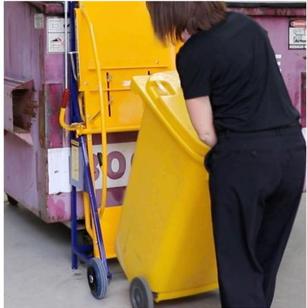
2. Push the wheelie bin forward to lock between the **wheelie bin hooks** and the **wheelie bin retainer** (refer to illustration below).
