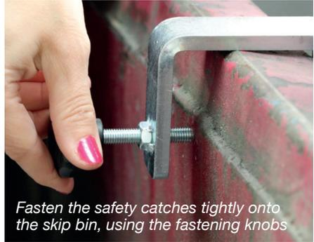
*Fasten the safety catches tightly onto the skip bin, using the fastening knobs*
