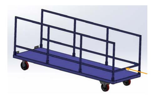
Assemble the cross bar between first and second side top and bottom.
