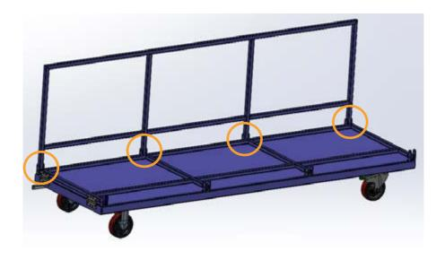
Using the 13 mm spanner and shifter, assemble the nuts and bolts (as shown in the four circled locations in the diagram above).
