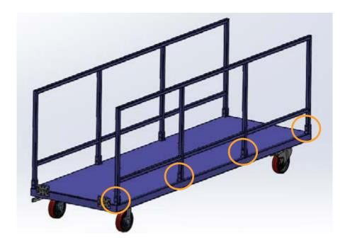
Using the 13 mm spanner and shifter, assemble the four nuts and bolts (as shown in the four circled locations in the diagram above).
