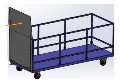
Assemble the ramp using the Allen keys and shifter.
